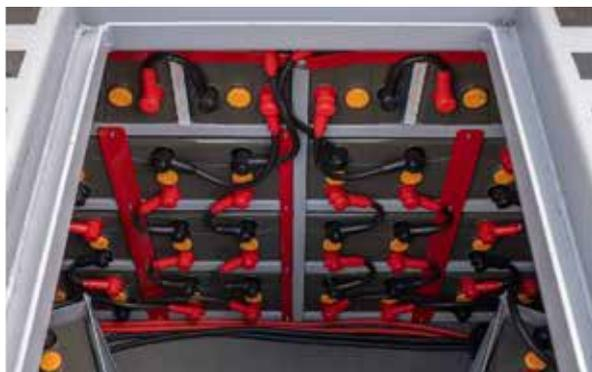
Through a complex Mastervolt Power management system, these batteries deliver power first and foremost to our electric propulsion motor, which spins at a very sedate 350-500rpm in "tickover" and around 1100 rpm when we're really going fast (no more than 4mph on the canals is allowed). It's a very spooky experience to those of us used to a noisy diesel engine to be travelling in a boat where the motor is pretty well silent.
